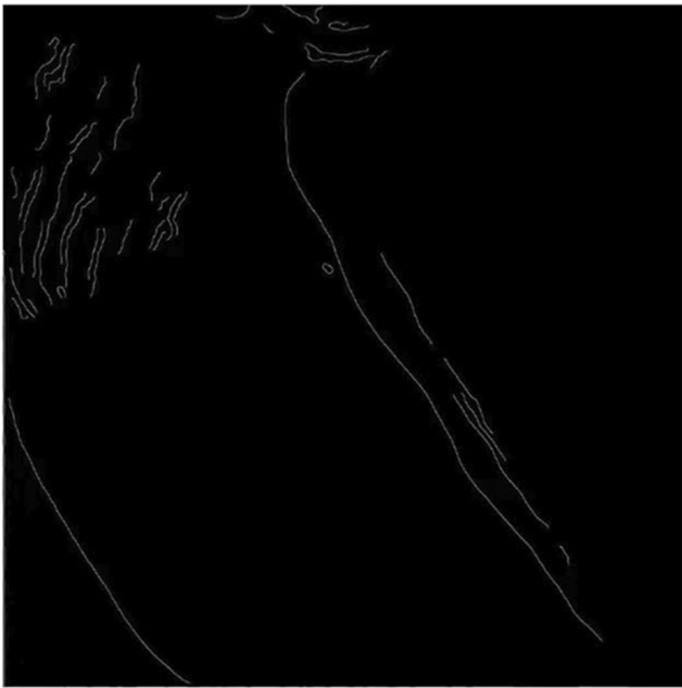
Fig. 8 The edge detection result of Canny operator in ocean internal wave SAR image
