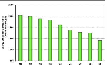
Furthermore, the application of the produced mortar samples to a wall surface is simulated. U-values of the structure formed by this simulation were determined. It is observed that composite mortars with pure pumice aggregate are much energy efficient up to 20.5%, according to the U-value results, when compared with the control specimen.
