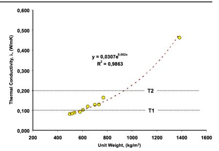
due to the fact that the pores forming the inner structure of the pure pumice make the heat difficult to transmit. Secondly, the mortars, produced by the pure pumice and tuff aggregates together, appear to be very resistant to heat and effective in energy saving.
