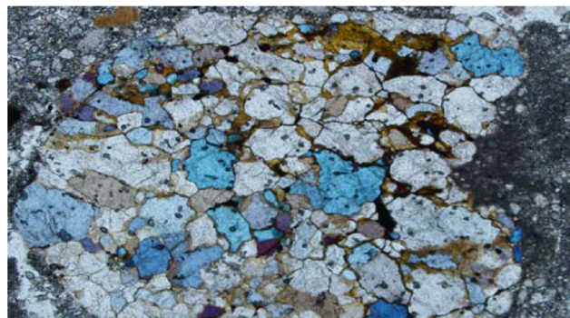
Fig. 4 Photomicrographs of calcrete from Rietfontein Farm, Limpopo Province, South Africa. (a) Plane-polarized microphotograph of calcrete from Rietfontein Farm - composed of fine micritic calcite lumps (light brown) surrounding quartz grains (white), and in turn surrounded by more micritic calcite mixed with fine iron-hydroxide (dark brown). The latter is cut by calcite veins (white). Field of view = 3 mm. (b) Cross-polarised micrograph of part of a veinlet of carbonate hosted by calcrete (Field of view: 200 \mu\text{m} across)
