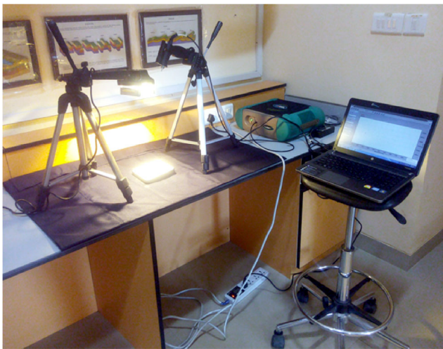
Fig. 8 ASD spectroradiometer used for spectral measurements in laboratory conditions
