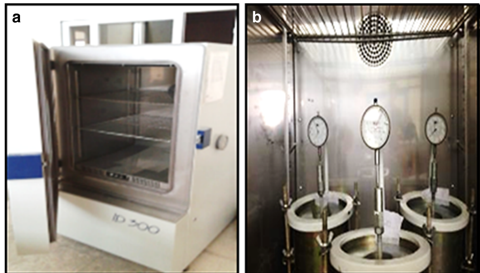
Fig. 1 Closed system freezing–thawing tests
