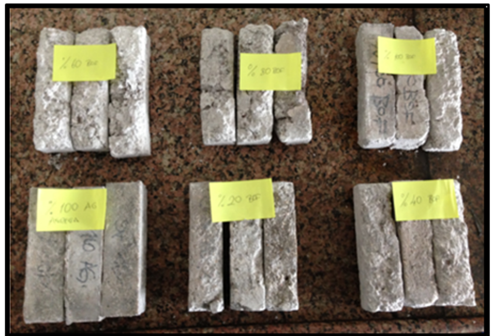
Fig. 6 The final state of the samples after freeze-thawing in saline (50 cycles)
