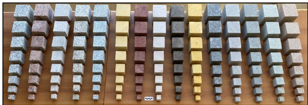
Fig. 1 Cubic samples with different edge lengths (between 3 and 10 cm) prepared for determining the sample size
