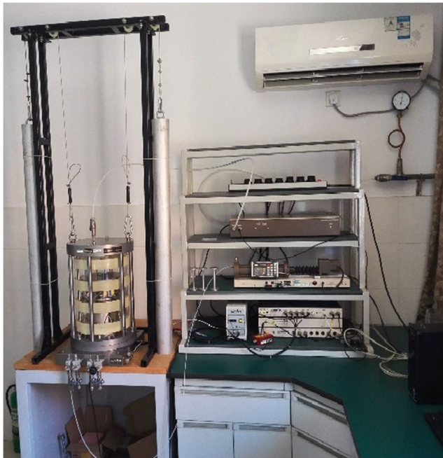
Fig. 1 GDS resonant column apparatus with specimen
