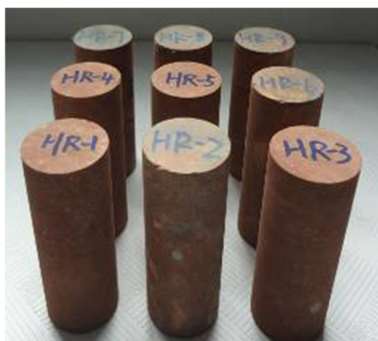
Fig. 2 Processed red sandstone specimens
