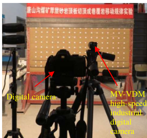
Fig. 6 Layout of the monitoring equipment on the similar simulation model
