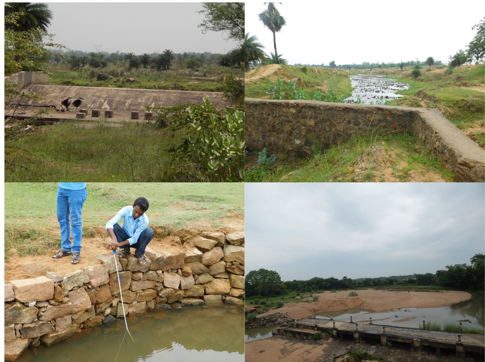
Fig. 6 Validation of the study and model through measuring the amount of soil deposition near the check dam
