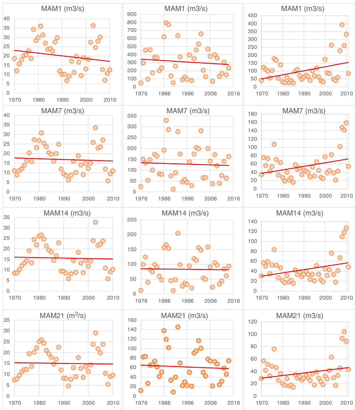
Fig. 6 Trends in maximum annual flows for the three gauging stations in the Mediterranean context: high flow indicators for the Evrotas catchment (left); high flow indicators for the Lonquen catchment (middle); high flow indicators for the Azzaba catchment (right)
