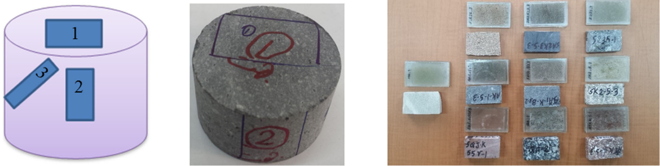
Fig. 1 Preparation of thin sections from core sample in three directions
