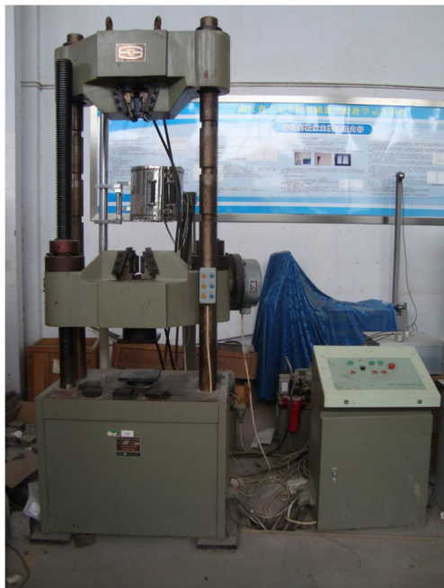
Fig. 3 WAW-600C universal testing machine
