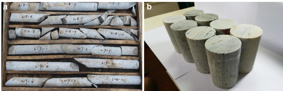
Fig. 1 Rock specimens. a Field cores. b Specimens
