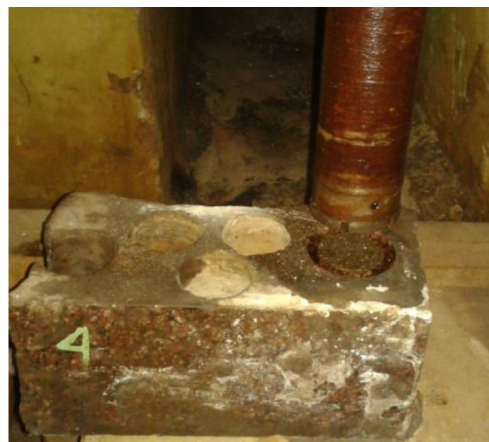
Fig. 3 Granite block used in a bench test drilling
