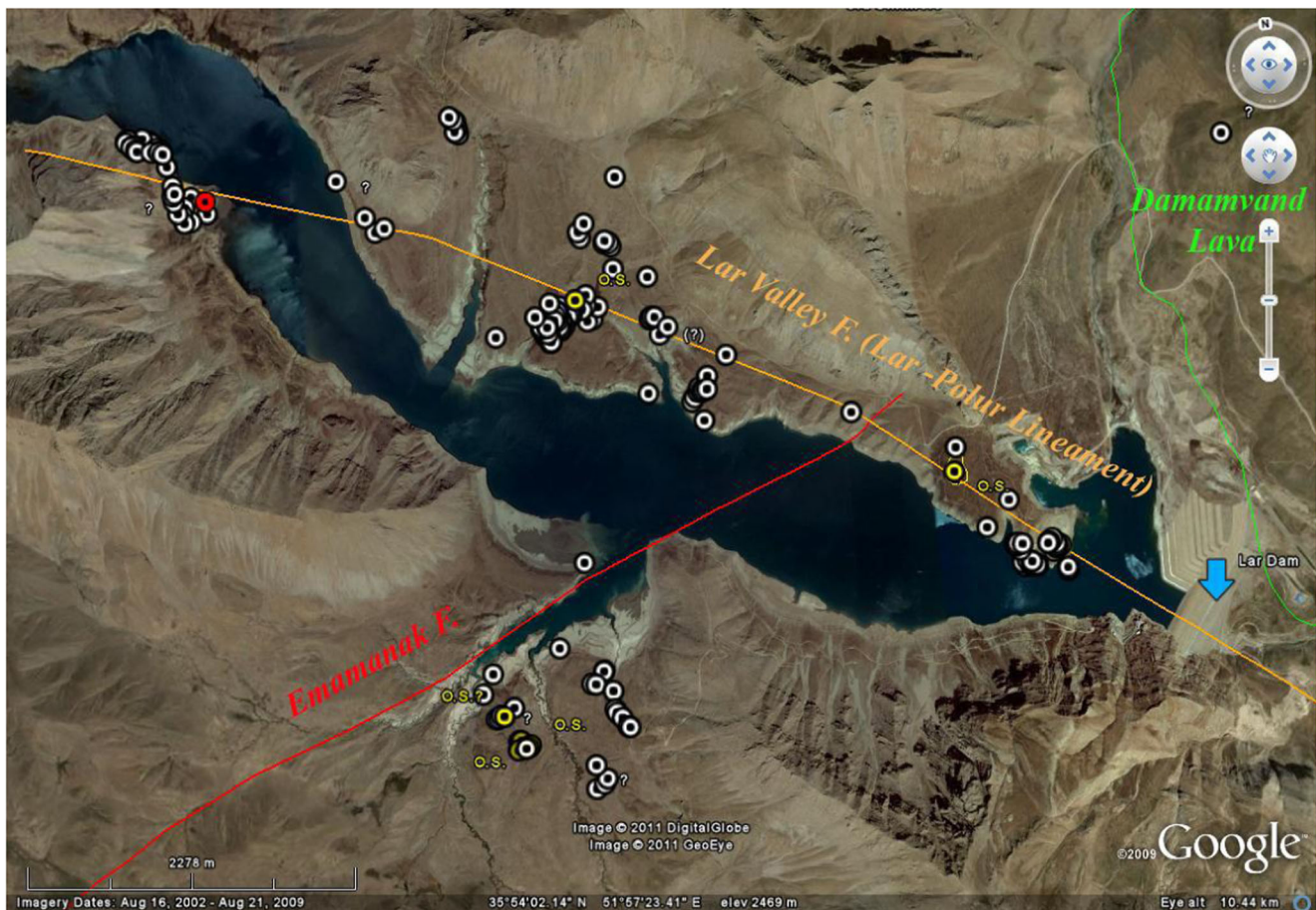
Fig. 4 Distribution of sinkholes in vicinity of Lar reservoir in the lake deposits. Circles indicate sinkholes
