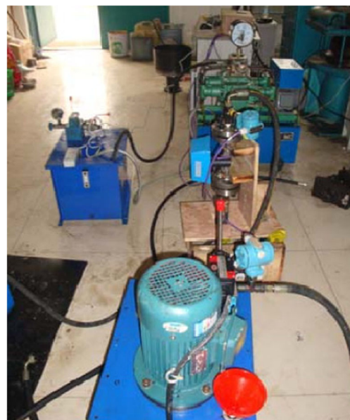
Fig. 9 Yao's seepage test system (Yao 2012)
