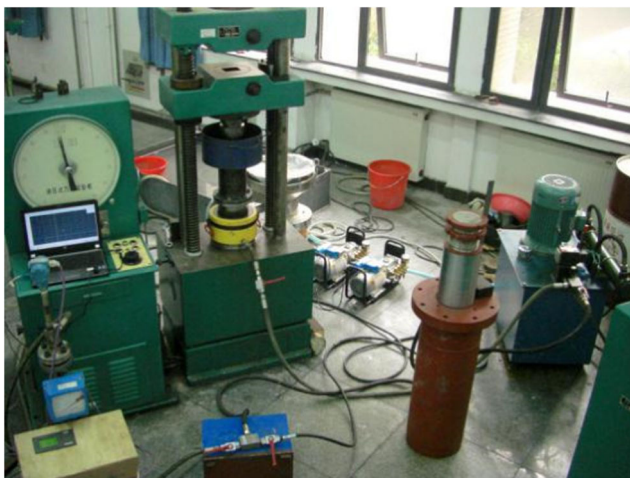
Fig. 13 The new seepage testing system for variable mass of fractured rock (Chen et al. 2014a, b; Wang et al. 2014c, d, 2016a, 2017; Kong et al. 2017a, b)
