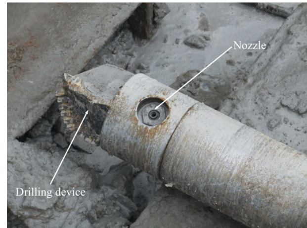
Fig. 1 a Schematic illustration of the jetting mechanism in the monitor (mono-fluid system). b Photograph of a monitor used for jet grouting
