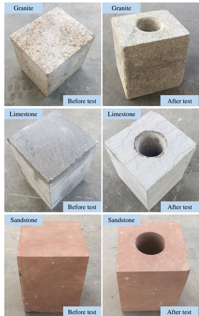
Fig. 6 Rock specimens before and after the test
