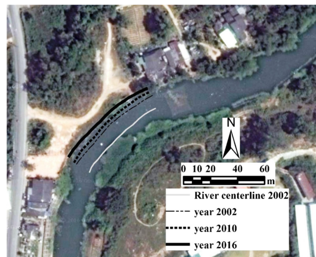
Fig. 4 Aerial photograph of U-Tapao River for bank retreat determination by analysis of aerial imagery
