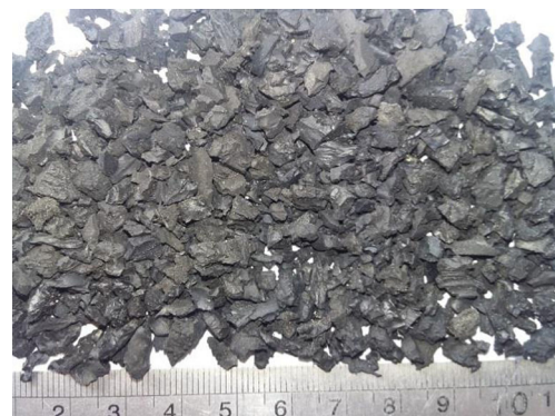
Fig. 4 View of granulated rubber with sizes in the range of 4 to 9 mm
