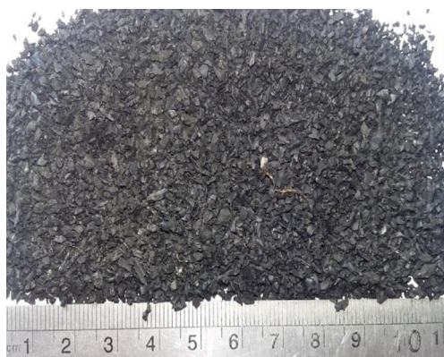
Fig. 2 View of granulated rubber with sizes in the range of 1 to 4 mm
