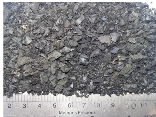
Fig. 3 View of granulated rubber with sizes in the range of 1 to 9 mm
