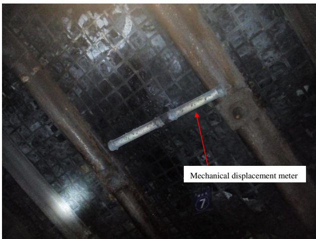
Fig. 5 Roof separation field-monitoring diagram
