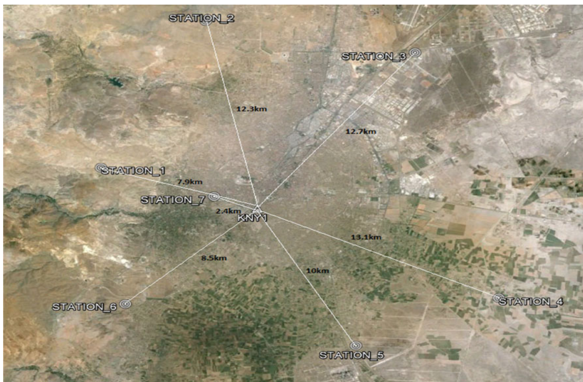
Fig. 2 Location of the test points w.r.t. the closest CORS station (KNY1)
