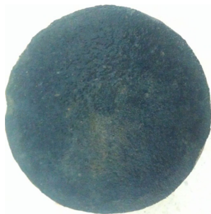
Fig. 13 Nano-copper materials assembled at the surface of soil sample S1 after hydraulic conductivity test
