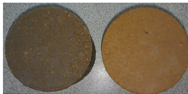
Fig. 2 Colour of soil samples after compaction: the light colour sample without nano-copper and the dark colour sample with 0.5 % nano-copper
