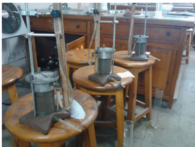
Fig. 9 Falling head permeability test setup
