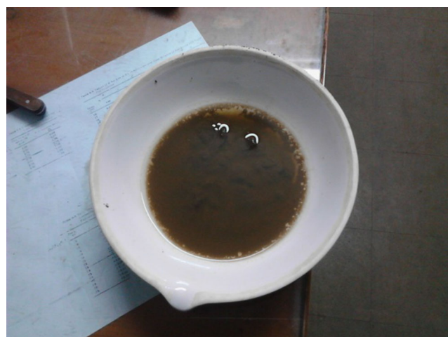
Fig. 5 Fifty grams of the soil soaked at 125 cm 3 of the sodium hexametaphosphate solution
