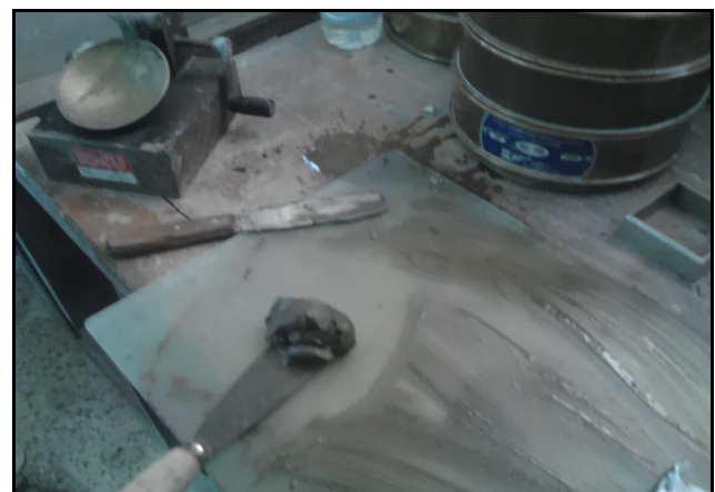
Fig. 15 Liquid limit apparatus used
