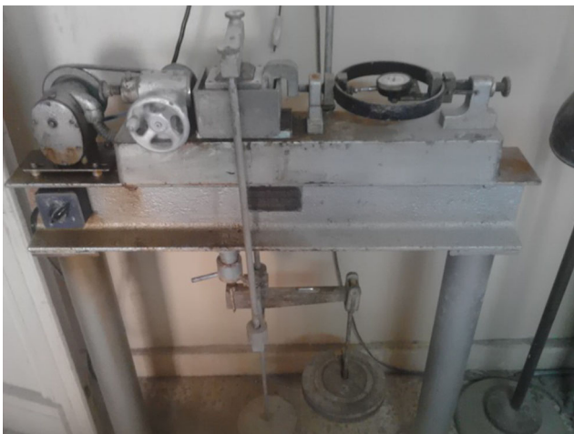
Fig. 17 Direct shear machine for sand
