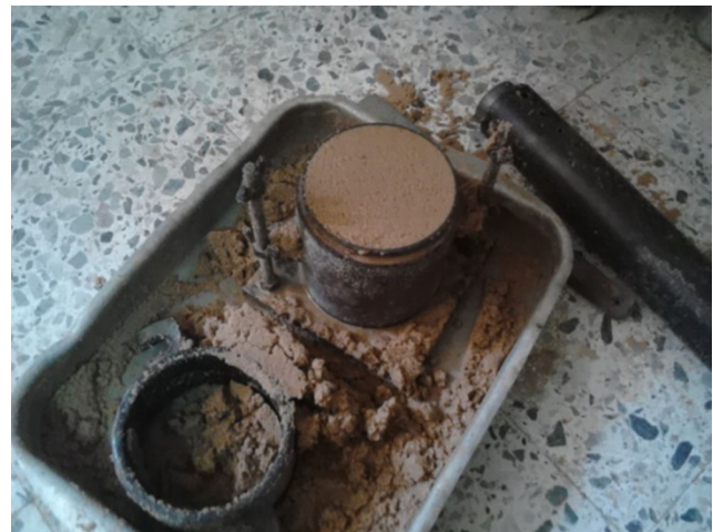
Fig. 8 Equipment for the proctor compaction test
