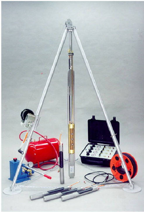
Fig. 3 A picture of applied equipment in the downhole test
