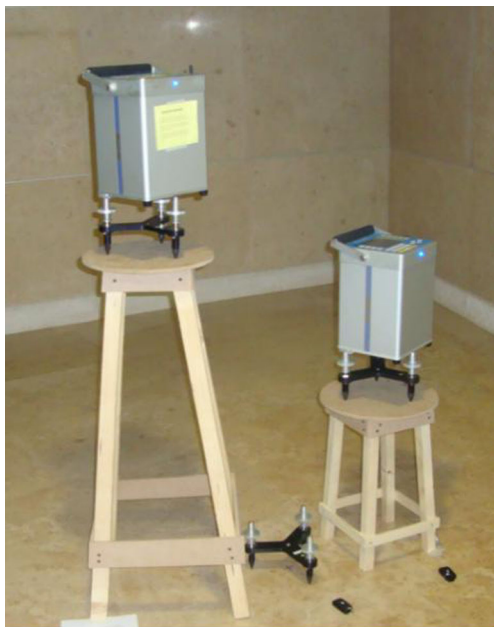
Fig. 3 Gradient measurements at 25, 75, and 125 cm by using CG5 mounted on tripods
