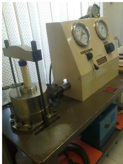
Fig. 3 Laboratory direct shear test setup
