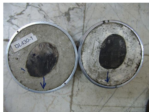
Fig. 4 Surface of natural joint after the shear test
