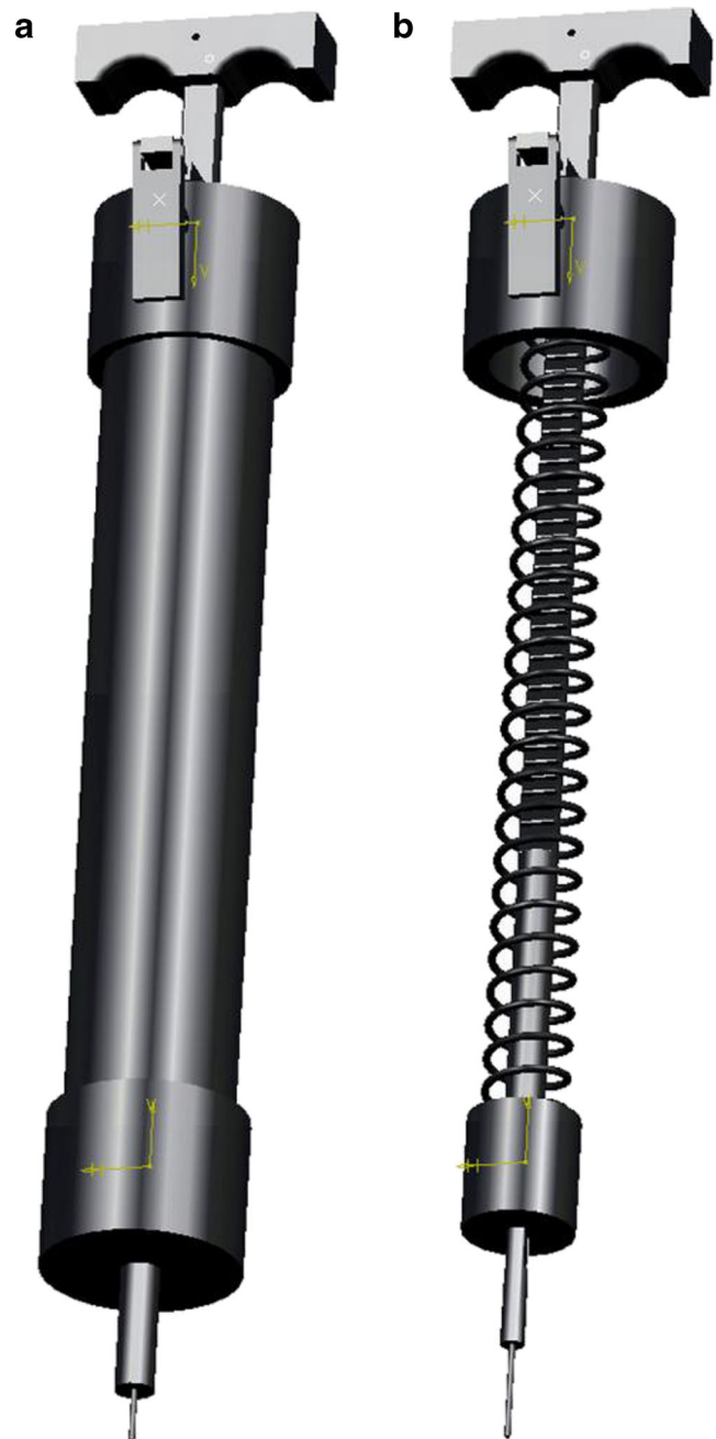
Fig. 3 Two different views of the 3D model of the dynamic needle penetrometer: a the assembled view, b the bare view
