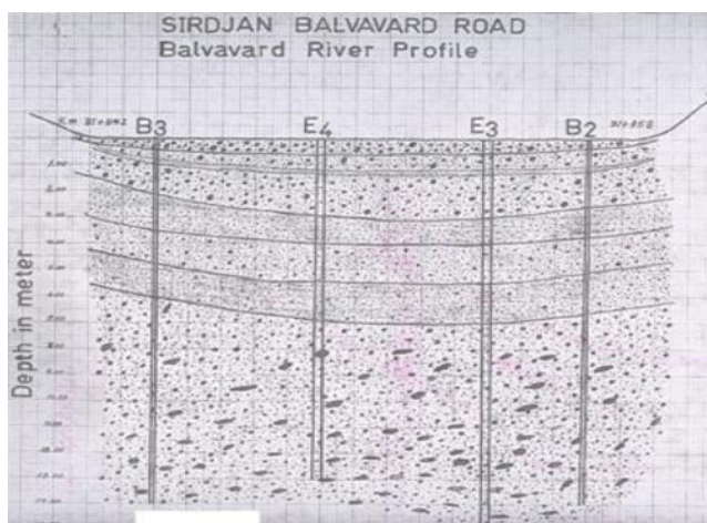
Fig. 9 Cross section of drilled boreholes
