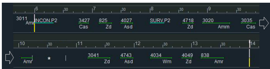
Fig. 1 A Gantt chart representation of a duty with assigned train control and platform control jobs
