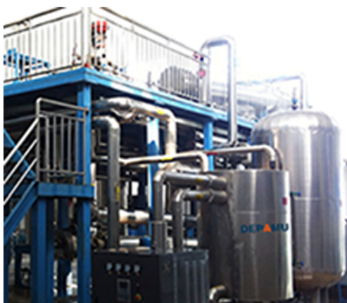
Fig. 3 Industrial SFE unit by DEPAMU Co. (China, picture reproduced with permission)
