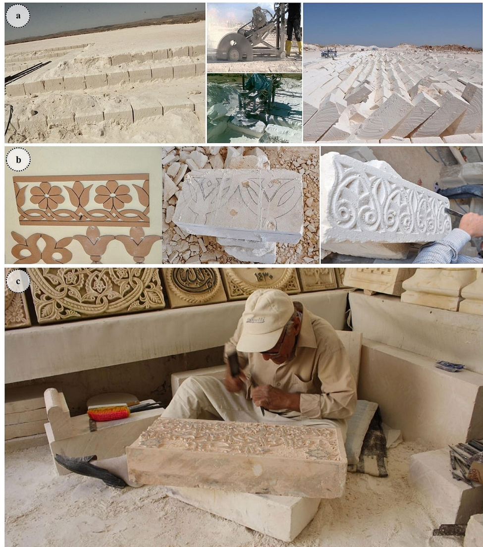
Fig. 8 Stone extraction and carving. (a) extraction of stone from a surface quarry; (b) Drawing and carving the desired pattern onto the stone surface by cardboard stencils and chisels; (c) A stone-mason practicing his art on the Mardin Stone ( http://tinyurl.com/mv48uaya )
