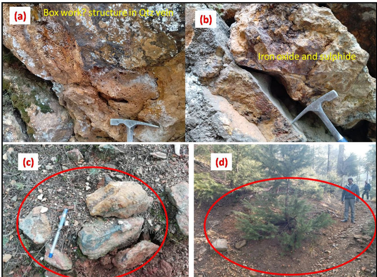
Fig. 12 Field photographs showing a, b box work alteration and oxidation in quartz vein c altered and leached boulders d gossan zone in the area
