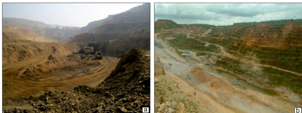
Fig. 28 a View of Jhamarkotra open cast mines. b East–west mining block exhibiting the benches on the foot wall at Jhamarkotra open cast mines, Udaipur
