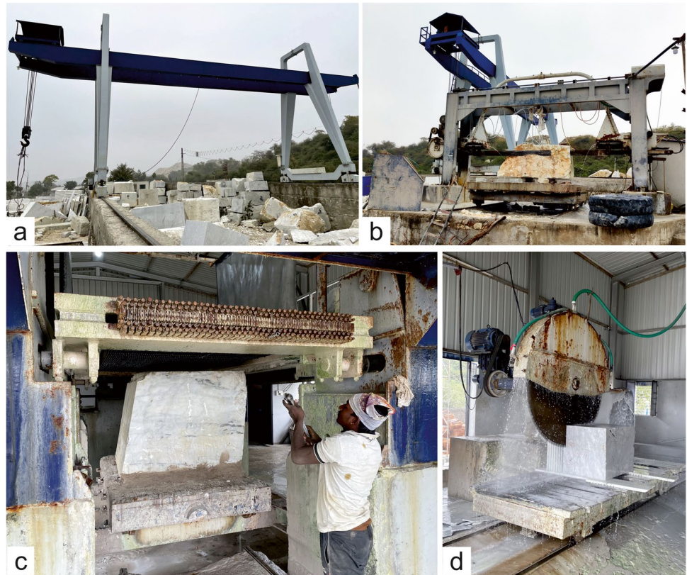
Fig. 5 Marble processing unit of RK Marble Pvt. Ltd. a Gantry crane used to unload marble block from the truck. b Block cutting machine. c Multi-wire cutting machine. d Circular saw used to cut the blocks of marble into slabs and tiles of variable sizes (photos by Sanchit Garg and Amritpaul Singh)
