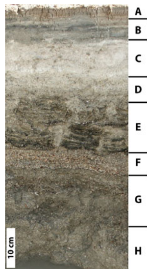
Fig. 3 Stratigraphic section through the Abu Dhabi coastal sabkha at N 24° 07.051, E 054° 02.994 (see Fig. 4a for location of section). A – halite crust and underlying carbonate mud, B – organic-rich carbonate mud, C – anhydrite with small gypsum crystals, D – gypsum lathes up to cm-scale, E – laminated microbial mats with sub-vertical cracks infilled with carbonate mud, F – cerithid gastropod lag, G – mixed carbonate and siliciclastic mud containing detrital clay and silt-grade quartz along with lenticular gypsum lathes up to 10 cm in diameter, H – siliciclastic mud with high organic content immediately overlying a hardground
