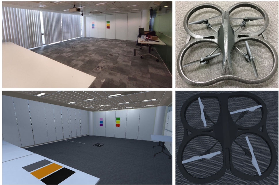
Fig. 1 The experimental room and the real Parrot AR.Drone 2.0 (top) next to their virtual replica (bottom) in Unity 3D. Participants' paths were recorded in the simulation (see Fig. 2), allowing the accurate assessment of proxemic preferences around the drone, in a safe and realistic environment
