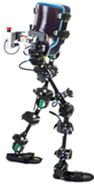
Fig. 1 Exo-H3 will be the device with which PROPELLING carries out its experiments (The EUROBENCH Project has made Technaid's Exo-H3 exoskeleton available for testing at their facilities. The Exo-H3 is the third version of Technaid's lower limbs robotic exoskeleton. Because it has been designed as a research platform, it can be adapted to fit differences in users' height and width while being compatible with a range of control algorithms. It thus allows applying the findings to a variety of robots on the market or under development. For more information, see https://www.technaid.com/landing-exo-h3 .)
