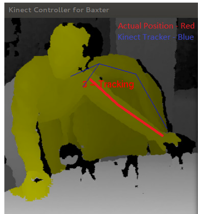
Fig. 3 Example of collecting kinematic data with markerless motion capture using Microsoft Kinect
