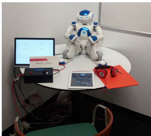
Fig. 4 Experimental setup for the embodied robot/power condition. Left to right: the tablet on which the participant could pick the correct answer in each trial (only for the power condition); envelope with the emotional face stimuli; the feedback box; the Nao robot; the tablet with instructions, movie and questionnaires; the folder with the information sheet and informed consent
