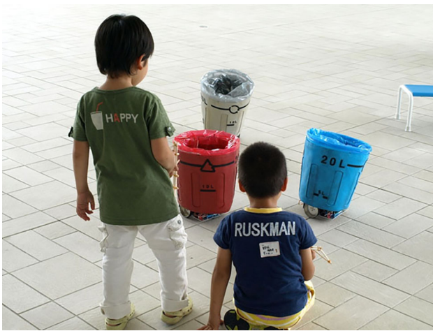
Fig. 1 The Sociable Trash Box exhibits helpfulness and politeness when it requests trash and then bows after receiving it. Reprinted by permission from Springer Nature: Springer International Journal of Social Robotics [56], © 2019
