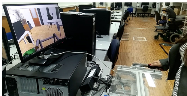
Fig. 4 A volunteer performing a run in the virtual environment using the ISR-AIWALKER’s HMI as input
