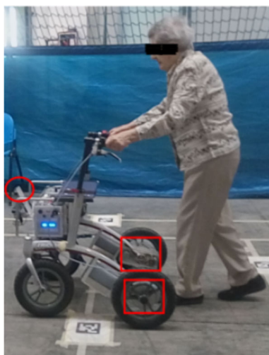
Fig. 1 Picture of the FriWalk prototype. The red circle emphasises the location of the webcam for QR-code detection, while the red squares indicate the mounting point of the encoders and the brushless motors. (Color figure online)
