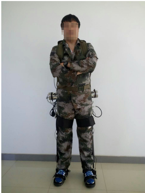
Fig. 2 Lower extremity augmentation device (LEAD) and pilot. From the point view of biomechanical consideration, exoskeleton can be seen as an anthropomorphic device which is parallel with the human body. In the design of exoskeleton, the comfortable locomotion is achieved by designing the number of DOF to be close to humans. Thus, our exoskeleton is designed as follows: the knee joint is actuated by a DC motorized ball screw; the hip joint in the sagittal plane is also an active joint, which is driven by a disk-type motor; the other joints are passive with elastic components due to the simplification of the control system and the consideration of total mass
