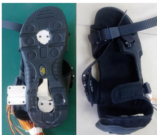
Fig. 4 Foot switch location. In order to maximize the sensitivity of the contact, the foot switches are mounted underneath ridges in the position of toe and heel respectively
