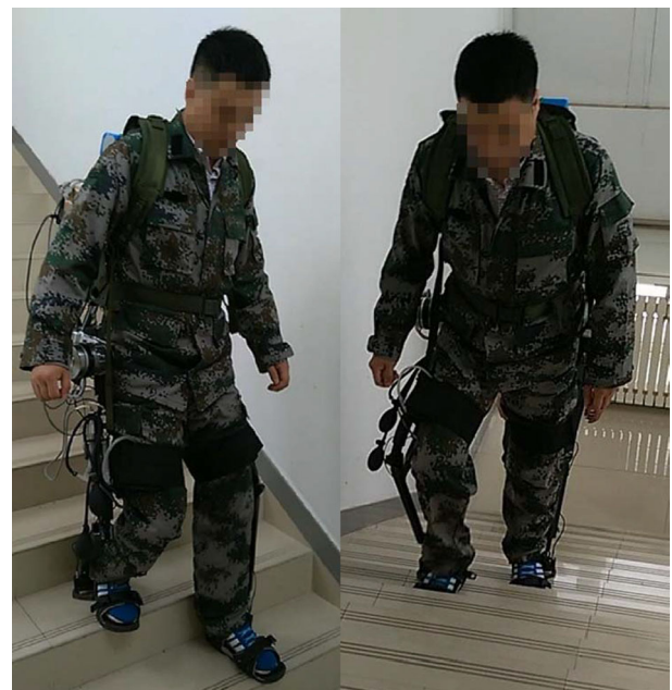
Fig. 13 Left graph: the pilot with exoskeleton goes downstairs. Right graph: the pilot with exoskeleton goes upstairs. We extend the experiments to going upstairs and downstairs
