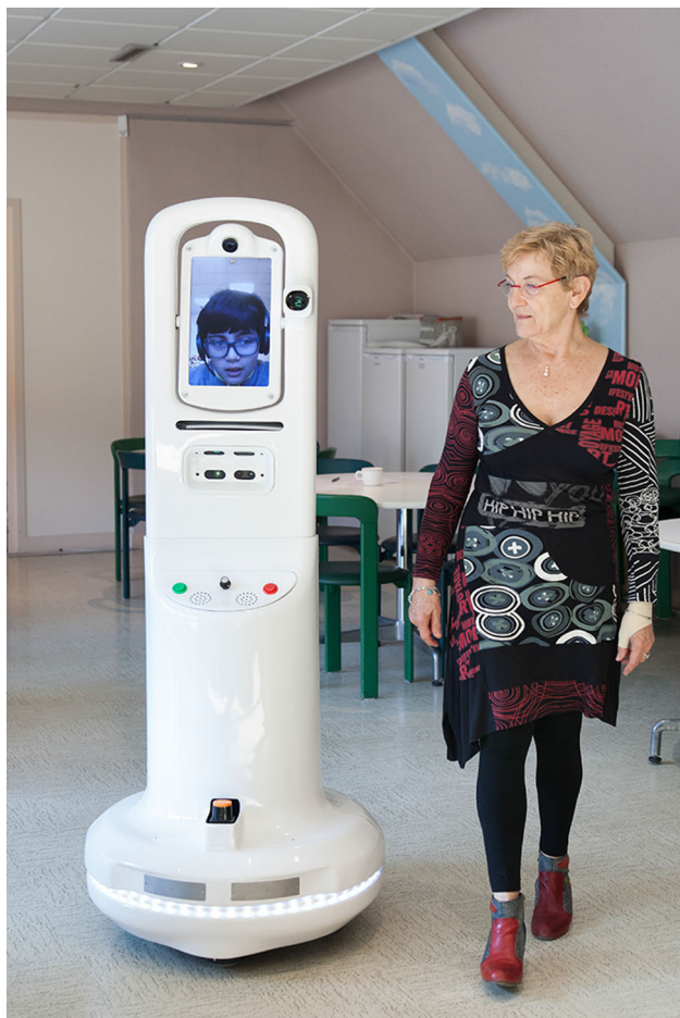
Fig. 1 Image of the telepresence robot developed in the TERESA project http://teresaproject.eu
