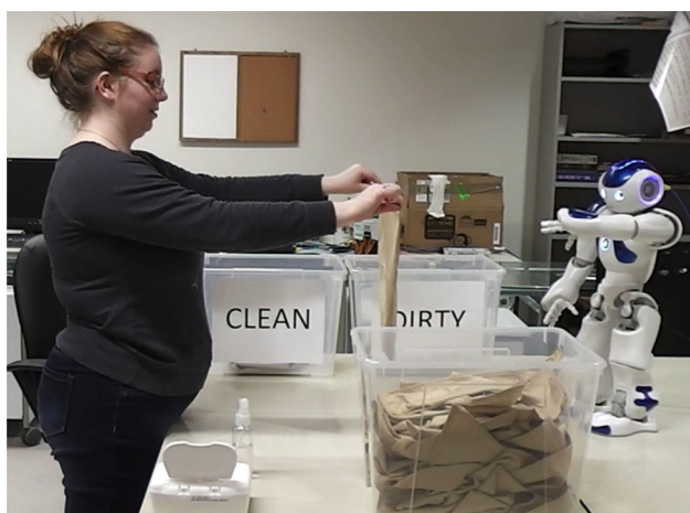
Fig. 2 A participant working collaboratively with a robot to sort pieces of laundered cloth. The participant leverages their manual dexterity to pick up a piece of cloth and hold it in front of the robot, while the robot ostensibly has a dirt sensor that can detect how clean the cloth is [42]
