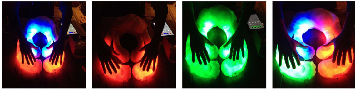
Fig. 2 Current prototype of +me , showing a sequence of possible light combinations. Lights and sounds behaviours depend both on the child, who touches the TWC, and on the therapist/caregiver who manages the input–output functions of the device
