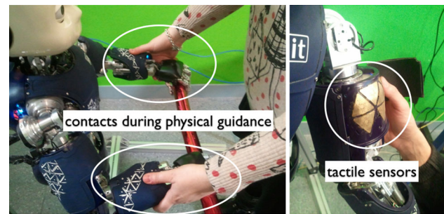
Fig. 4 Demonstration on how to safely grab the robot arms for kinaesthetic teaching in the assembly task: the hands of the experimenter grasp the robot forearms on a part covered by the skin. On the left , the distributed tactile sensors underneath the cover
