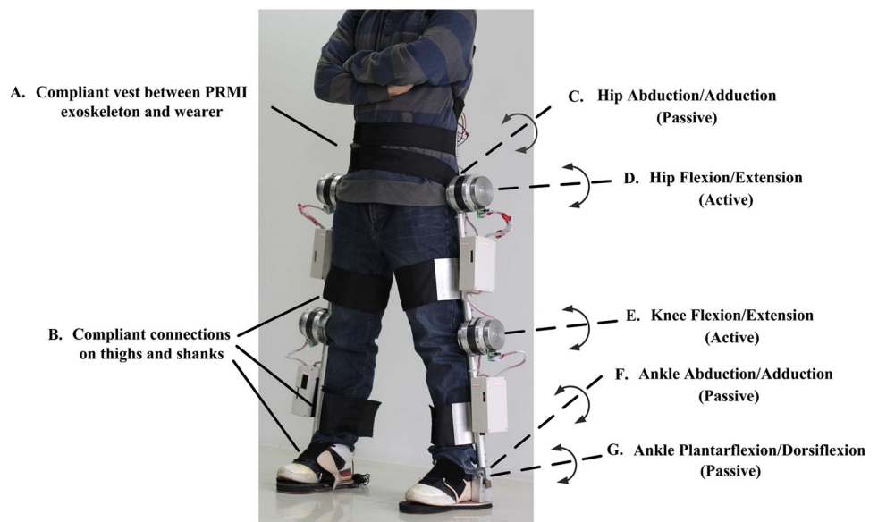
Fig. 7 Mechanical structure of the AIDER exoskeleton, showing the degrees of freedom
